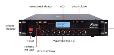
When one of the lights in the first row turns orange, it means that the corresponding channel has failed. The light directly below it will then illuminate, indicating that the backup channel is taking over the failed channel.
